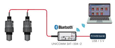
Instruments with HART<sup>®</sup> connectivity can be linked to a PC via Bluetooth<sup>®</sup> using a **UNICOMM** HART<sup>®</sup>–USB/Bluetooth<sup>®</sup> modem (SAT–504). The USB power bank connected to the **UNICOMM** modem can power the entire setup.
